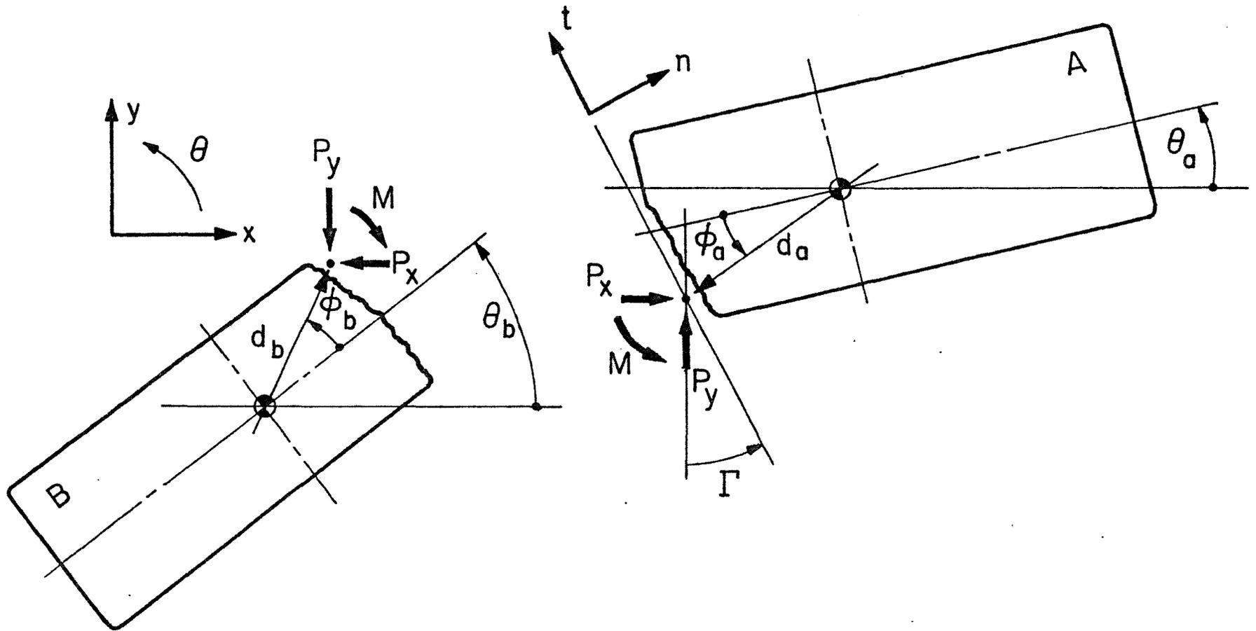
Figure 3. Free Body Diagrams for Planar Impact Model.
