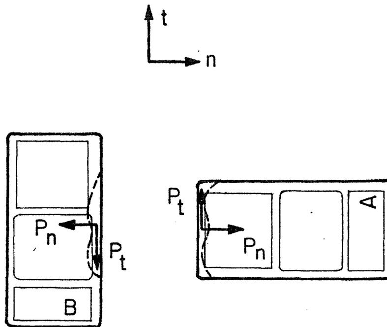
Figure 2. Free Body Diagrams of Vehicles for Direct Colinear Impact.
