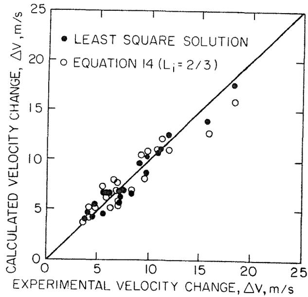
Fig 4 Comparison of Calculated Velocity Changes with Experimental Values
