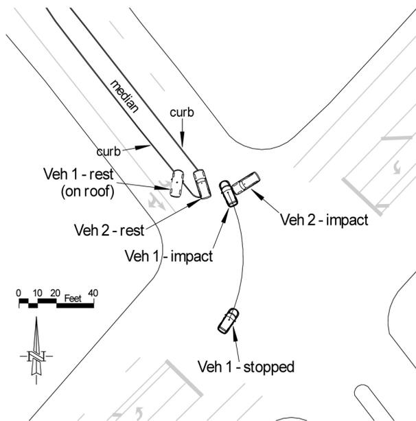
Figure 3.1. Scale crash diagram for Example 3
