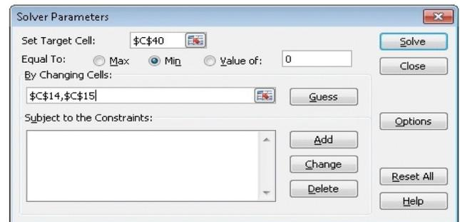
Figure 4.2. Input to Solver routine for minimization of  $Q$  (cell C40, Fig 4.1) in order to find the vehicle initial speeds (cells C14 and C15).
