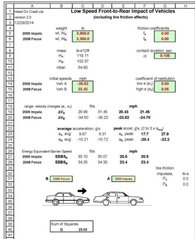
Figure 4.1. Spreadsheet with results of the least-square reconstruction of Example 4. Shaded cells are for known input values for an analysis; unknown input values can be found using the *What If* feature for a reconstruction when output information is known or specified.
