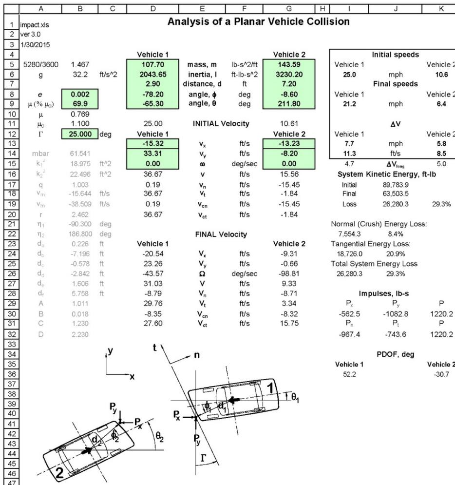
Figure 3.3. PIM solution spreadsheet for Example 3
