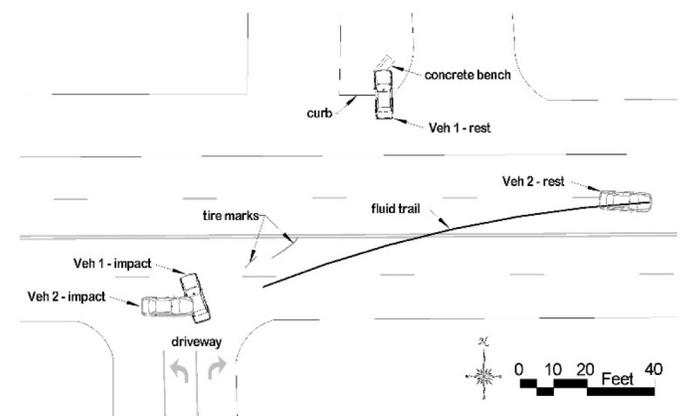
Figure 1.1. Scaled crash diagram for Example 1
