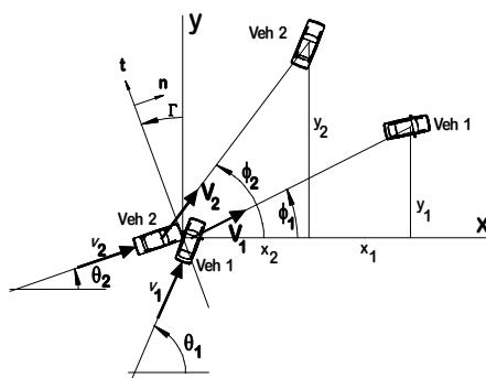
NOTE: This method is valid only for oblique collisions. In-line, collinear collisions ( $\theta_1 = \pm \theta_2$ ) can give inaccurate results.
